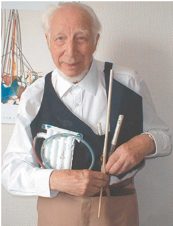
Fig. 3 Willem J. Kolff demonstrating the Wearable artificial lung. The whole unit is assembled on a vest. It has two components: a mi-LVAD and an oxygenator. The mi-LVAD consists of a concentric double-lumen cannula (held apart for better demonstration). A short wide cannula in the left ventricle has holes through which blood is sucked out and sent through a four-channel oxygenator (white area, right side of vest). Oxygenated blood is delivered into the aorta through the long cannula, the tip of which sits in the aorta. The mi-LVAD can be inserted transapically.
