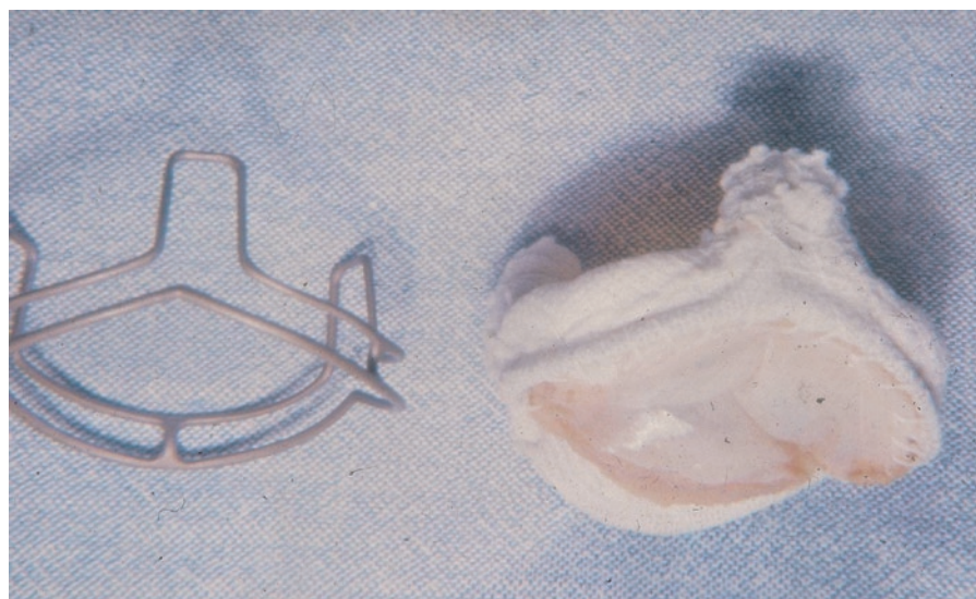
Figure 1 First (homemade) glutaraldehyde-treated pig valve implanted in human. Left, Teflon-covered stainless steel stent used to support the valve, preventing its deformation during implantation. Right, stent covered with Dacron fabric to facilitate fixation and host-tissue incorporation. The porcine valve has been sutured into the stent preserving a full motion of the leaflets, avoiding fibrous incorporation. From ref. 6.
