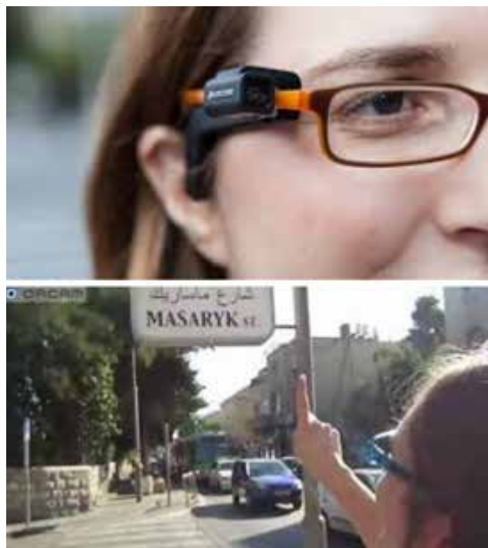
Figure 7.8. The Orcam device. A small camera mounted to the temple of the glasses acquires the visual scene and “speaks” the text at which the patient points. In this example, the patient is pointing at the sign that reads MASARYK St., and the Orcam device speaks the word.
