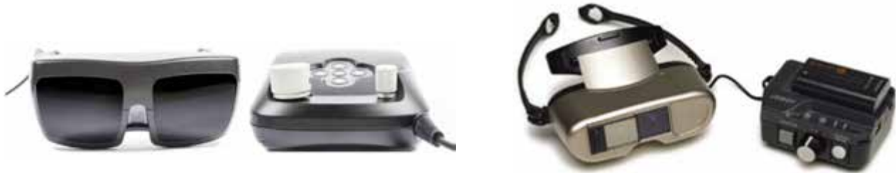
Figure 7.4. Left: Video goggles marketed by eSight. Right: A mobile visual aid called the "Jordy" marketed by Enhanced Vision. Both models suffer from a small field of view and cumbersome knobs to adjust parameters.
