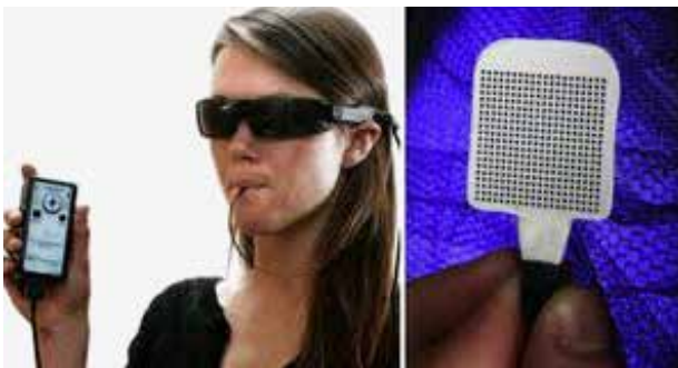
Figure 7.6. The “Brainport” generates a tactile display as an array of vibrating “pixels” placed upon the tongue. Patients have shown remarkable prowess using this device to perform sporting activities, for example. (Photo courtesy of Wicab.)
