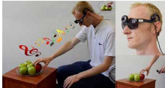
Figure 7.7. Images captured by the video camera are converted into the sequences of sounds representing brightness or color of various parts of the scene. (Photo courtesy of Amir Amedi Lab.)
